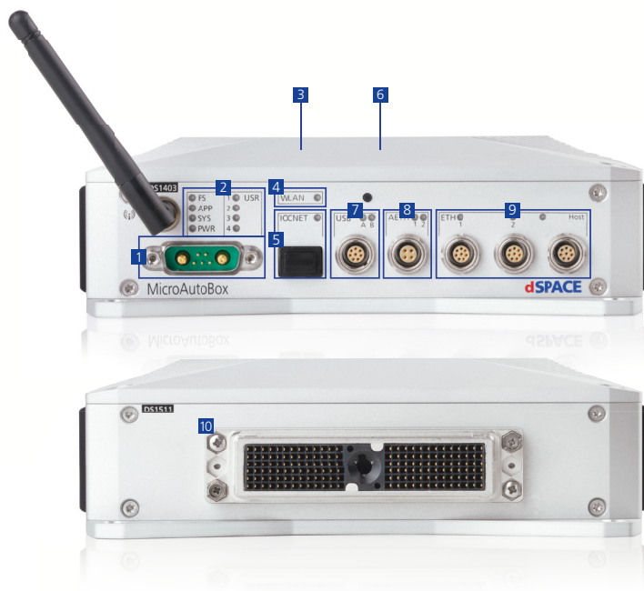
Figure 1: Compact design with all interfaces relevant for automotive applications – the new MicroAutoBox III (here: MicroAutoBox III 1403/1511).
