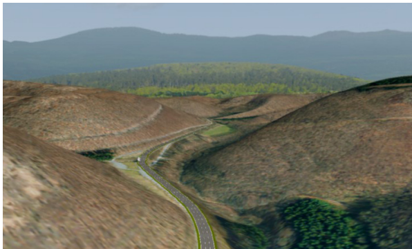
Terrain model generated from satellite images and digital elevation data with embedded road based on GPS data and generated by ModelDesk.
