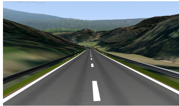
Resulting visualization from driver's perspective including enhancements such as delineator posts and barriers.
