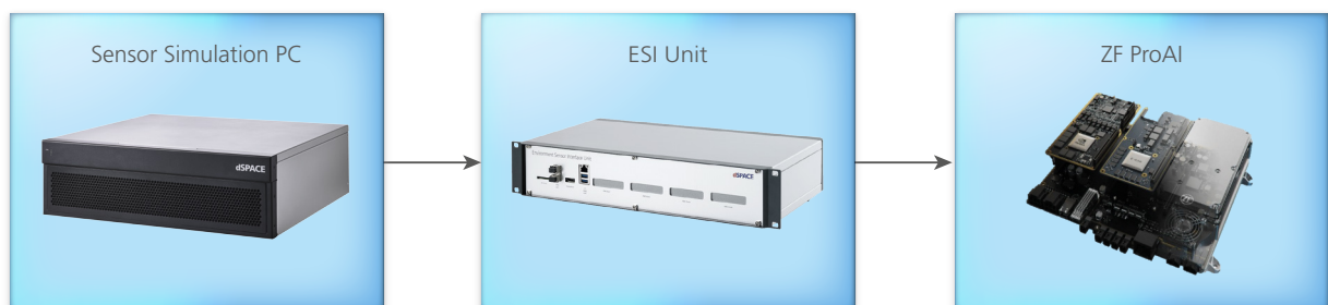
The sensor simulation platform: The sensor data is simulated on the Sensor Simulation PC. The Environment Sensor Interface Unit (ESI Unit) is used to provide electrical signals in the same way as real sensors would.
