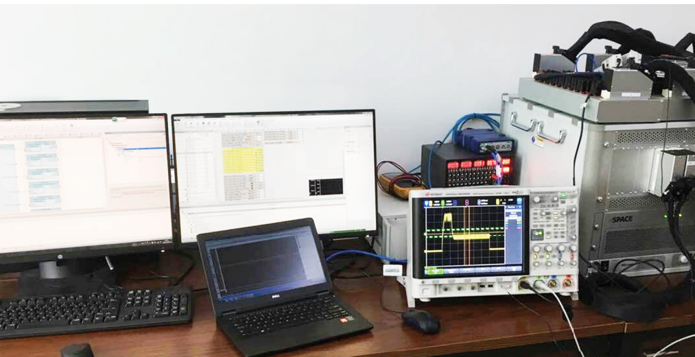
Figure 2: The dSPACE test bench consists of a SCALEXIO simulator and a drive load box. The compact system has a small footprint. It is easy to operate from the host PC. The signals are measured with an oscilloscope.
