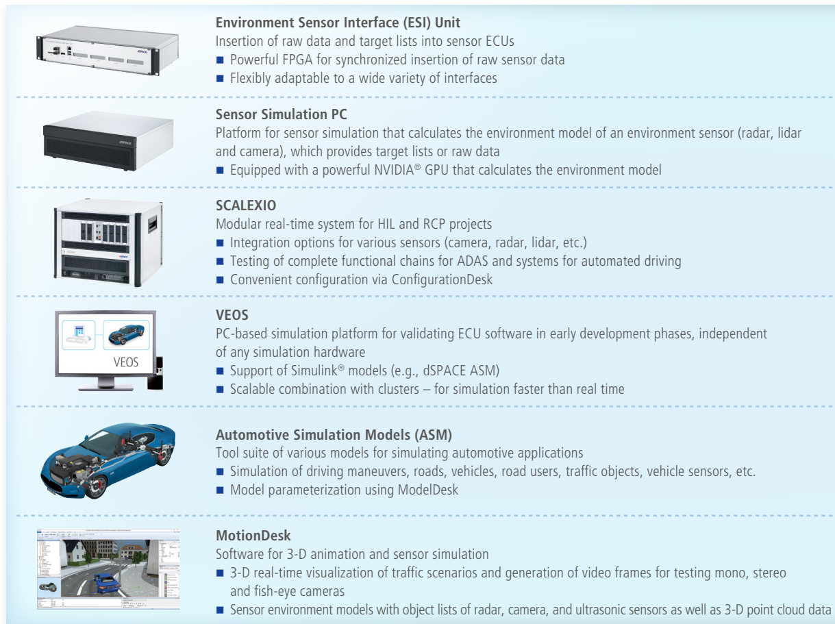
Figure 2: Overview of key products of the dSPACE tool chain for sensor simulation.
