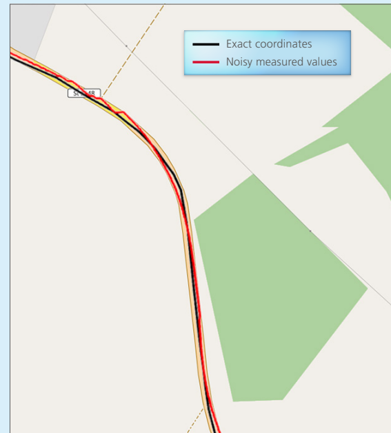
Left: The exact coordinates (blue) of a test track are determined from the noisy measured values (orange) by means of map matching. Center: For comparison, the route as displayed in OpenStreetMap. (Contains information from OpenStreetMap ( openstreetmap.de ), which is available here under the Open Database License (ODbL) opendatacommons.org/licenses/odbl/ .)
