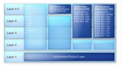
A wealth of possibilities: Automotive Ethernet provides multiple software layers above the physical layer. They can be used for an application-specific combination of protocols, such as SOME/IP, AVB, and TSN.
