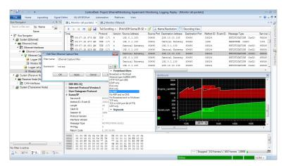
Monitoring: The Bus Navigator in dSPACE ControlDesk can be used for easy monitoring and recording of Ethernet traffic. The built-in Ethernet filter makes it possible to limit data capturing to individual Ethernet package types. The Time Cursor in ControlDesk lets you easily compare recorded Ethernet communication with other buses and measurement data.
