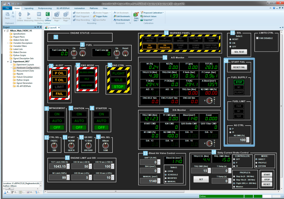
Figure 4: The graphical user interface of dSPACE ControlDesk clearly displays the extensive control and display parameters for the engine tests.
