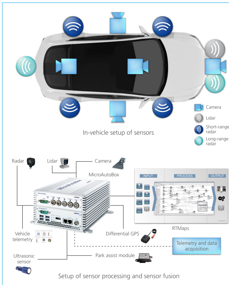
To merge various sensor signals and perform the relevant processing algorithms in real time, RTMaps and MicroAutoBox took over crucial roles.
