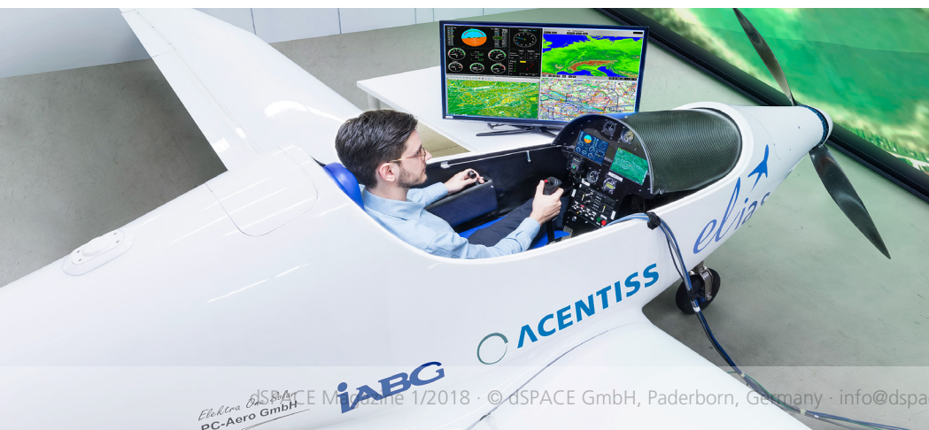
Figure 1: Aircraft-in-the-loop simulation is used for comprehensive testing of the flight control algorithms on the ground.
