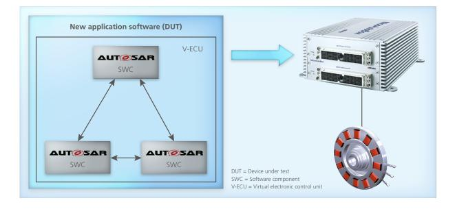
The controller software was migrated to an AUTOSAR-compatible structure, which let FAW use it in the vehicle.
