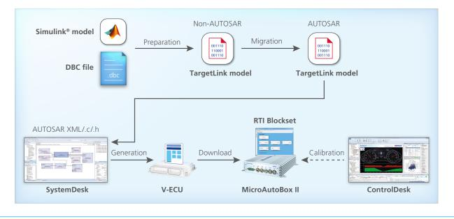
Migration process for the controller software of an AUTOSAR-compatible ECU. The controller software can be tested in the vehicle using the prototyping system.
