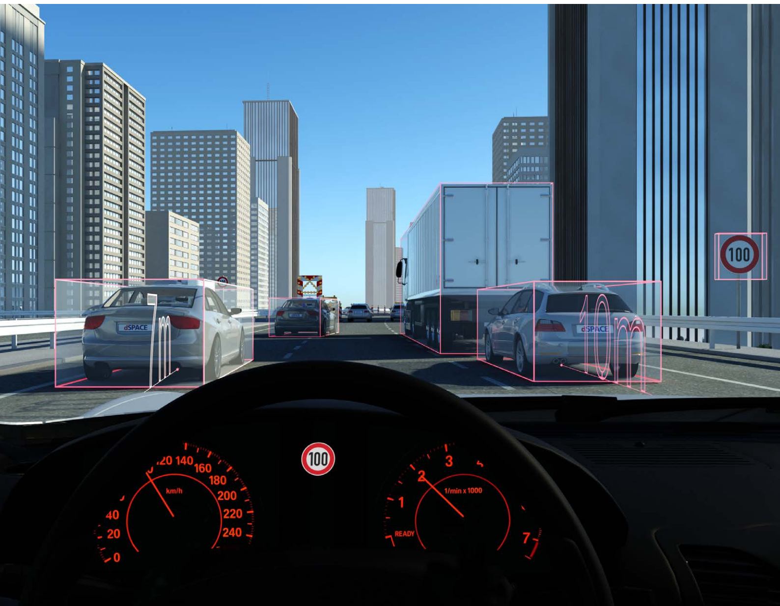
Detection of surrounding vehicles and traffic signs with the sensor model of ASM Traffic.
