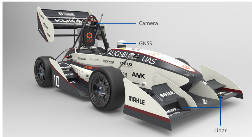
The autonomous vehicle by the Augsburg University of Applied Sciences is equipped with a global navigation satellite system (GNSS) and captures its environment by using a camera and two lidar sensors.
