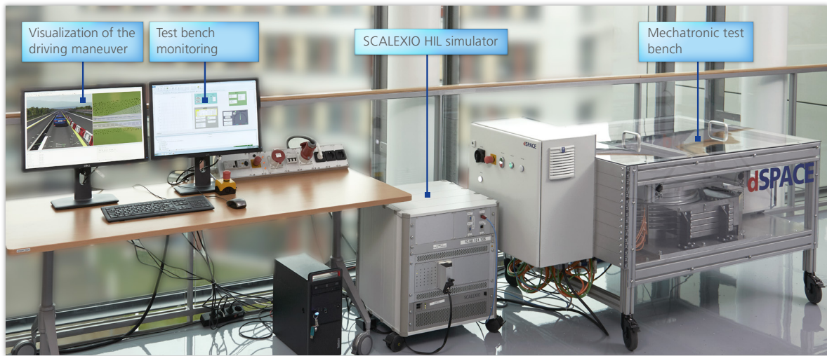
Figure 1: An overview of the radar test bench.
