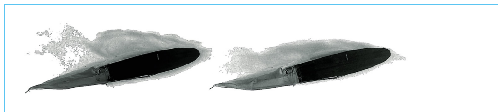
Figure 4: The visualization of the airflow shows the effect of adjusting the wing shape to stall conditions. Left: Strong formation of vortices due to no adjustment. Right: Wing adjustment almost completely suppresses vortex formation.
