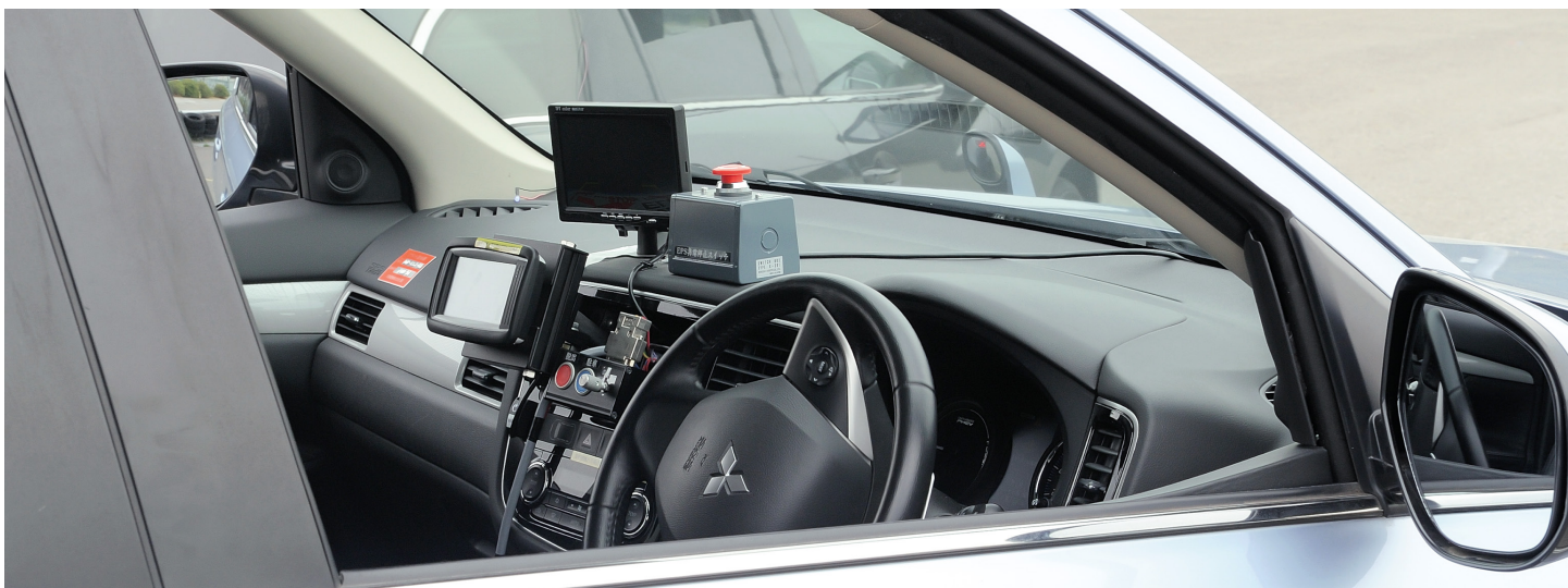
Dashboard of the vehicle equipped with the autonomous driving features.
