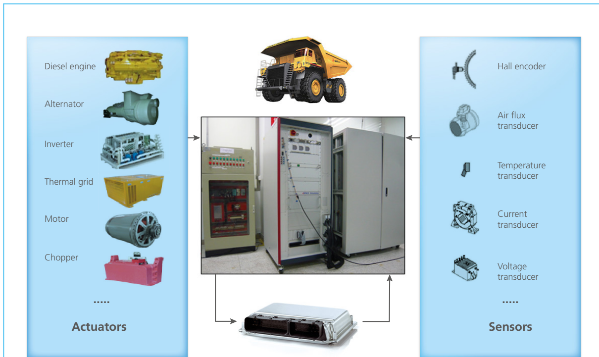
Virtual vehicle: The turn-key dSPACE Simulator Full-Size replicates the SET230’s entire sensor system (on the right) and actuator components (on the left). This lets the engineers at SANY test the basic control strategies together with the other vehicle components at an early stage, without any expensive test drives with a real dump truck.
