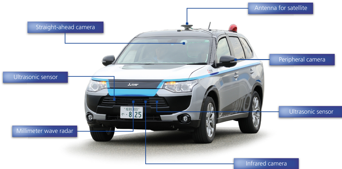
Overview of the sensors for autonomous driving.
