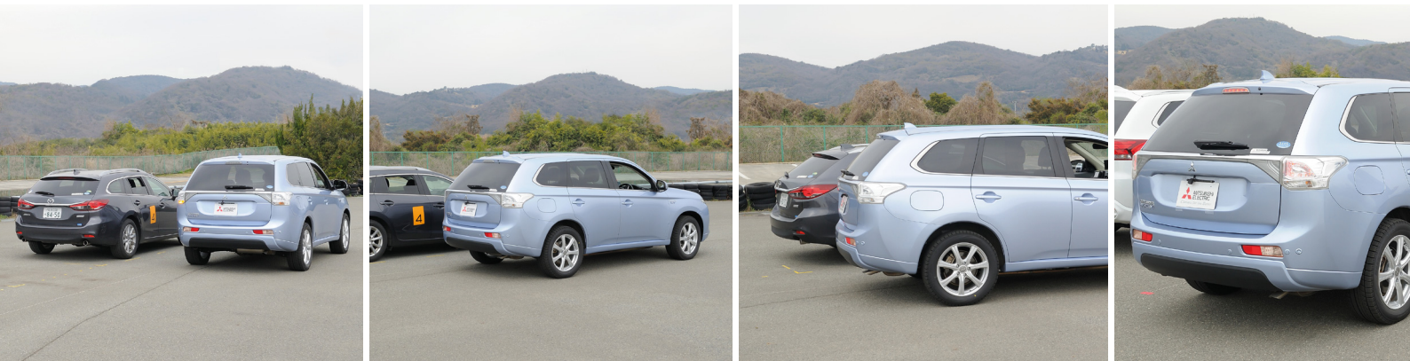
Autonomous parking initiated with an external device, e.g., a smartphone.
