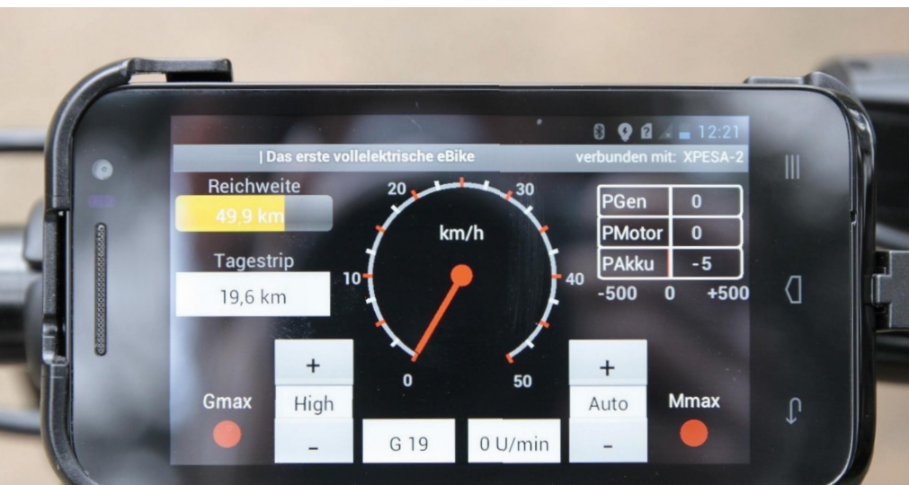
Figure 2: The user interface of the smartphone, connected via Bluetooth.
