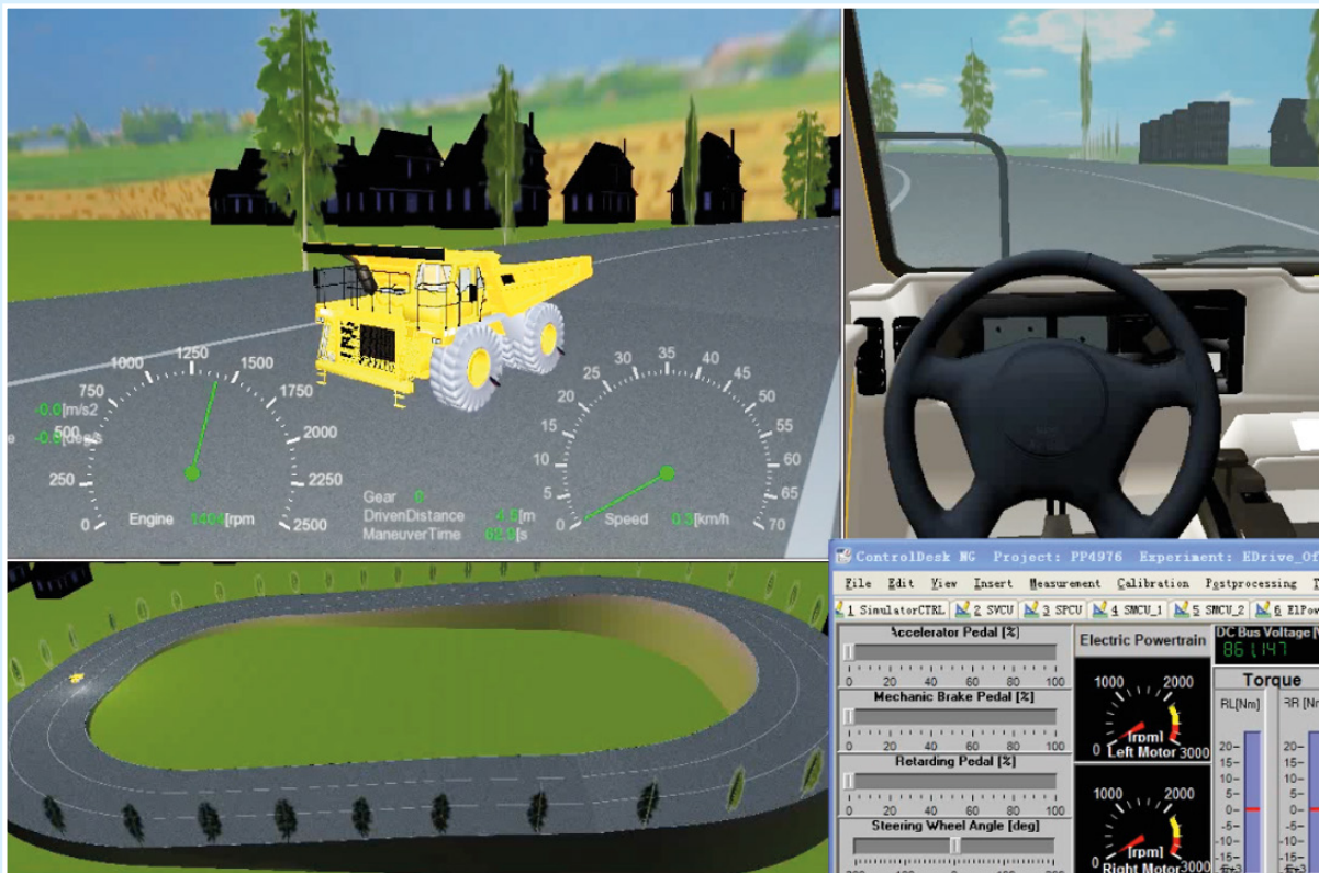
Clear visuals: In dSPACE MotionDesk, SANY engineers can replicate the driving maneuvers and scenarios simulated on the HIL system in a clear 3-D online animation. This lets them visualize the effects of parameter changes in real time.
