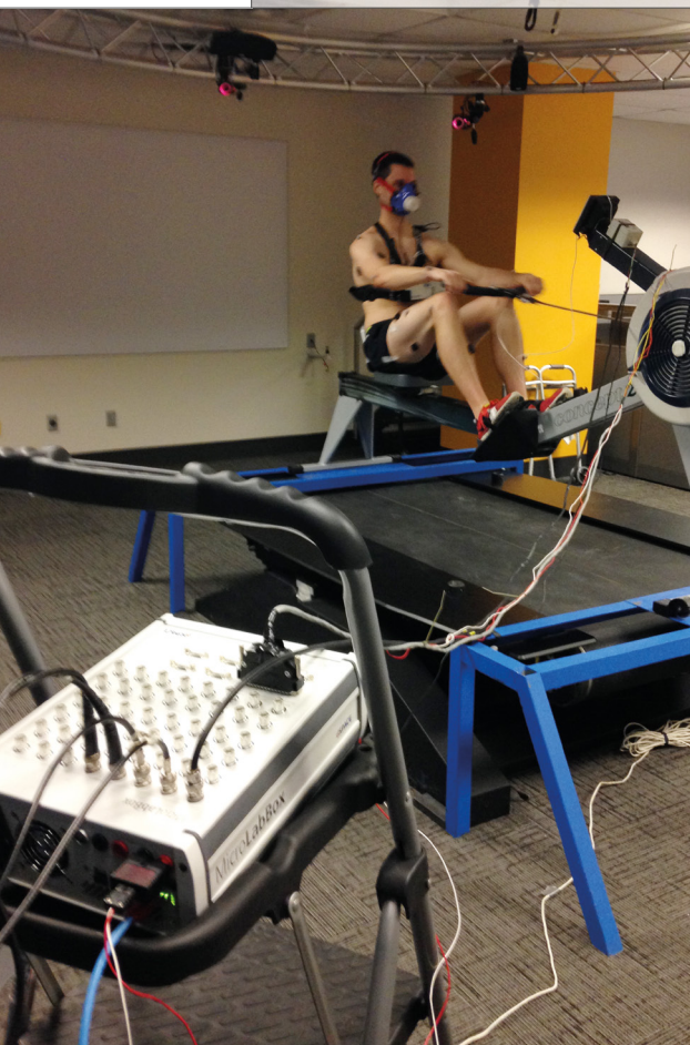
Figure 3: During a trial, dSPACE MicroLabBox (left picture) collects 16-channel electromyography (EMG) data and machine mechanical data at a sampling rate of 1 kHz. A separate system collects motion data using visual markers (shiny spots) and metabolic data. Data from all systems is synchronized by offline postprocessing.
