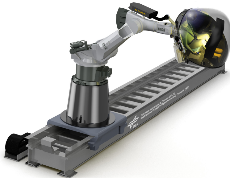
Figure 3: To increase the operational space, a linear axis is used for the DLR Robotic Motion Simulator (RMS).
