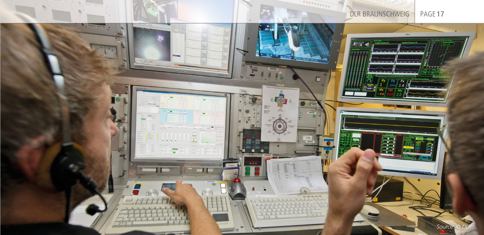
Control and monitoring systems for the wind tunnel test, with two ControlDesk layouts (on the right).
