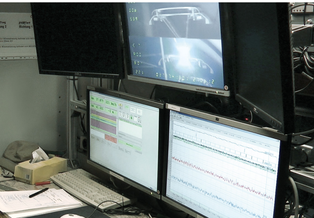
Figure 5: Test drives can be used to demonstrate how effectively the new pantographs prevent electric arcs.
