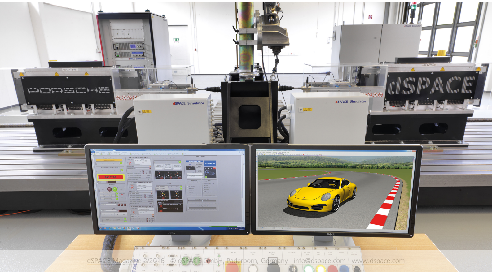
Figure 4: The mechatronic test rig, including the operator workstation with ControlDesk for controlling the tests (left) and MotionDesk for visualizing the driving maneuvers (right).
