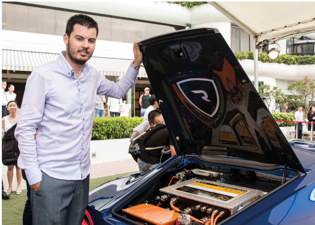
Mate Rimac, inventor of the Concept_One, beside the opened vehicle rear showing the power distribution unit.
