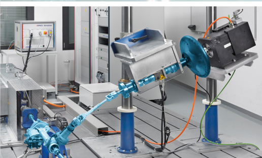
Test bench for steering systems (single-sided linear motor).
