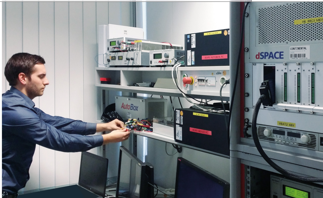
Figure 2: One of the HIL test rigs at Continental in Regensburg.
