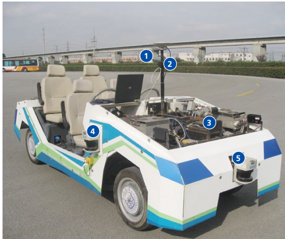
Figure 1: For orientation, the prototype vehicle uses GPS, camera, laser radar (lidar) and a millimeter wave radar.
