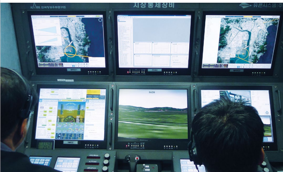
Figure 4: The ground control station transmits commands to the aircraft and displays all the aircraft's instruments. Virtual 3-D graphics give a virtual cockpit view, which is useful for monitoring the aircraft's situation in case the pilot-view camera malfunctions.
