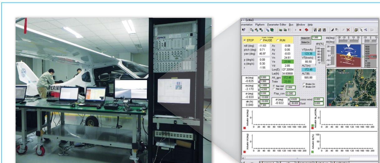
Figure 2: The dSPACE Simulator executes virtual test flights in the laboratory. The test and experiment software dSPACE ControlDesk (shown on the right) is used to monitor all the experiments and insert failures.
