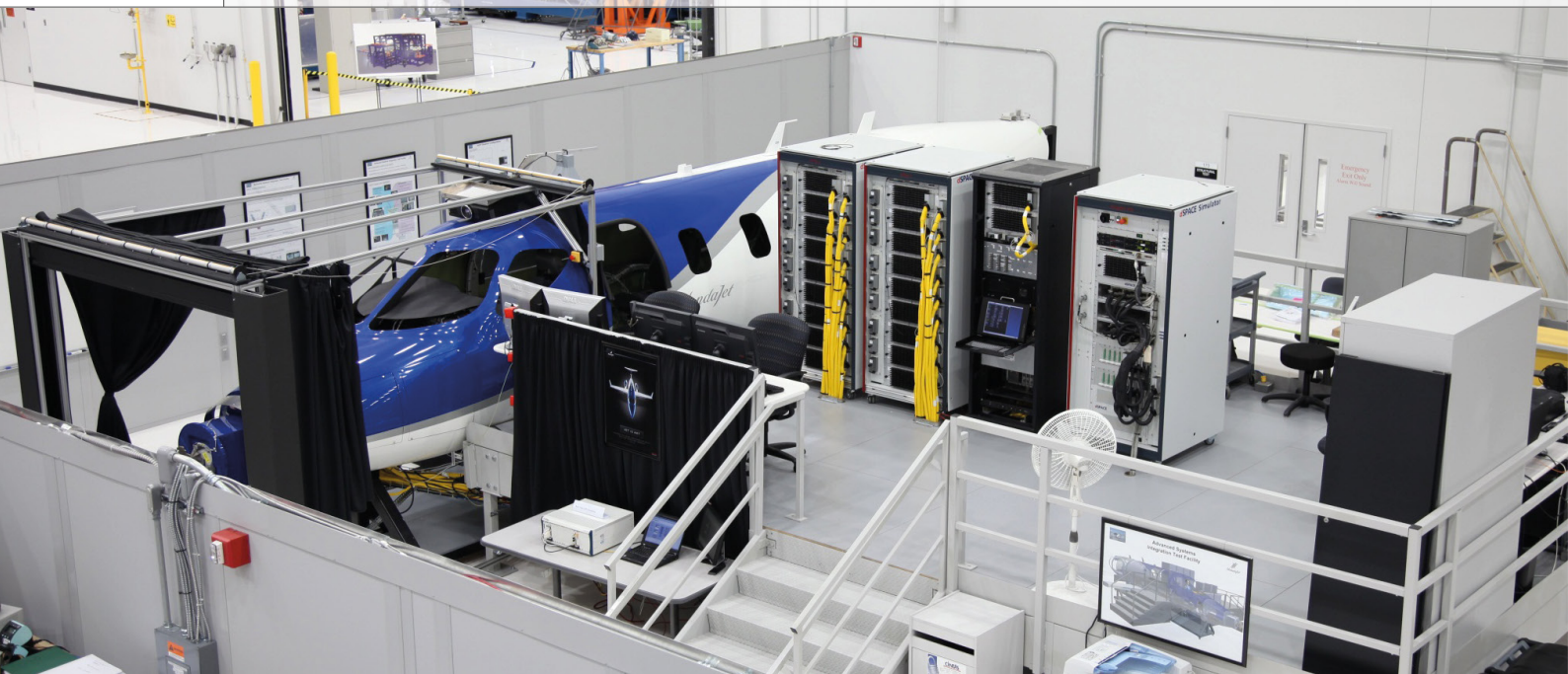
The test lab including the iron bird (left) and the three dSPACE HIL simulators (center).
