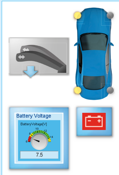
Figure 1 (left): This is how signal-based testing works: In this example, the behavior of the turn signal is tested at a low onboard voltage (7.5 V) and after the turn-signal lever was activated.
