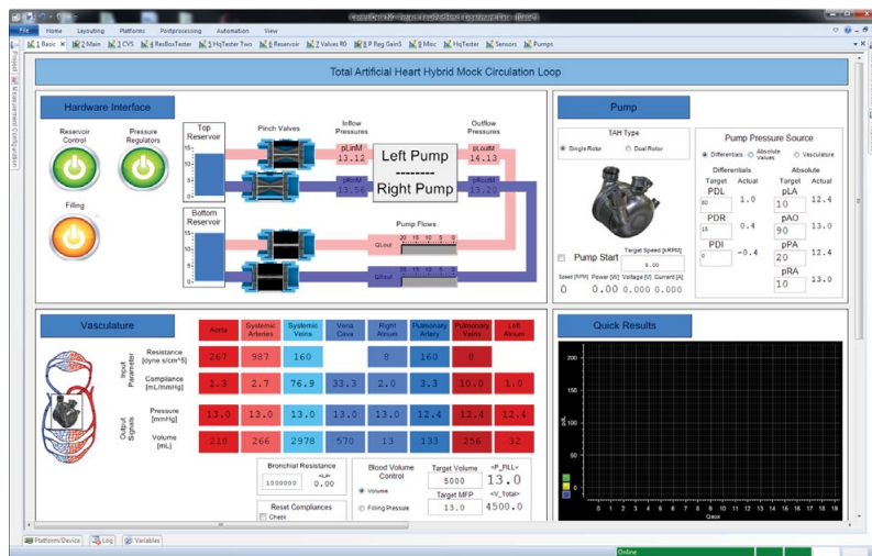
Figure 3: The dSPACE experiment software ControlDesk Next Generation provides the central user interface and serves to record data, change parameters, and graphically displays different system states.
