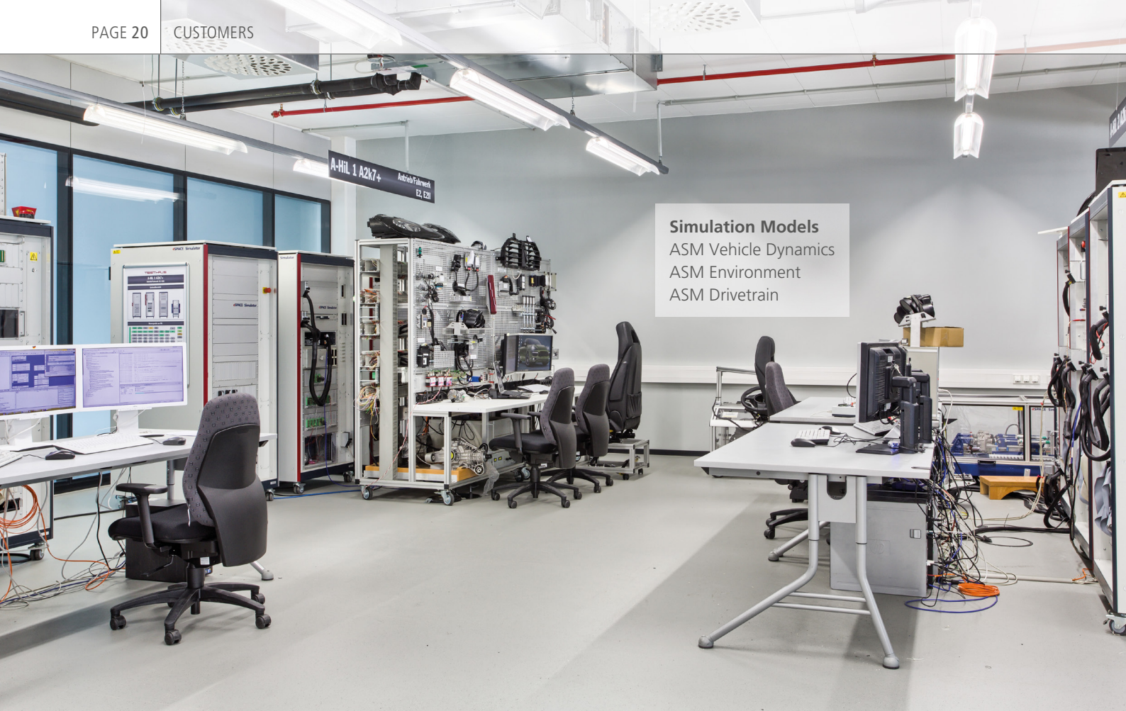
Figure 1: HIL test benches for validating the drive/chassis applications. A setup for installing ECUs and for integrating real components (throttle valves, injectors, transmission valves, actuators for the electronic parking brake, radiator shutters, etc.) is located at the center back.
