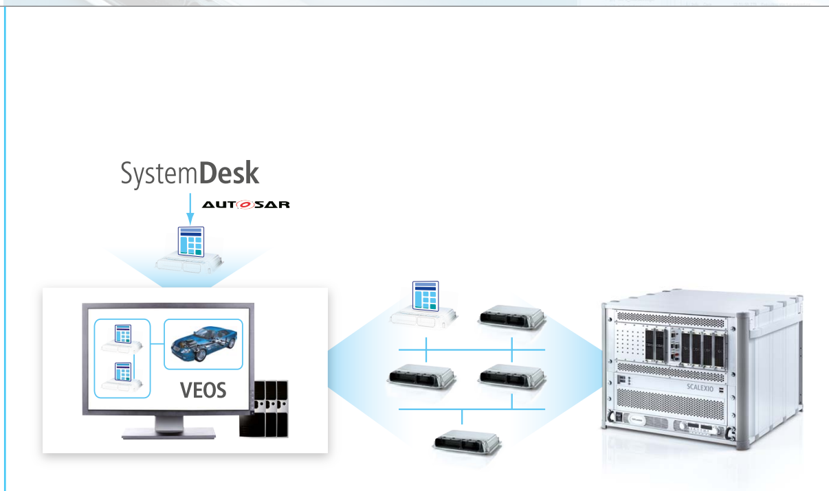
Figure 3: Virtual ECUs can run on dSPACE VEOS and on SCALEXIO. The same software is used to configure and handle them in both cases.
