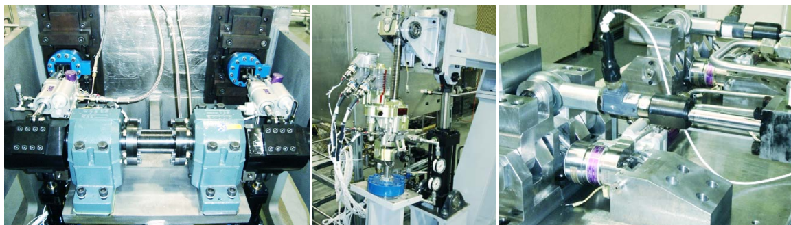
Figure 7: Actuator test rigs for testing commercial flight control systems (left: rudder actuator test rig; middle: HSTA test rig; right: spoiler actuator test rig).
