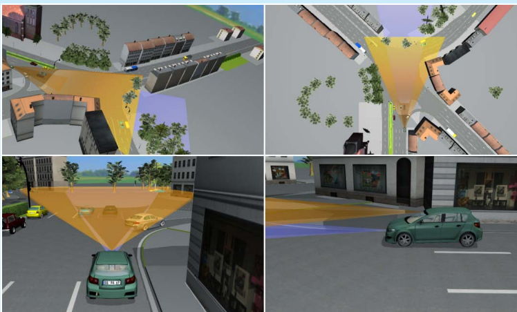
Figure 4: The intersection from different viewpoints in MotionDesk. The view cones of the monocular camera and the radar sensor are visualized in orange and blue respectively.
