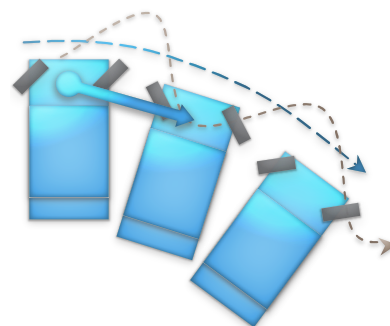
Figure 1: Example of a side maneuver to the right: The vehicle automatically moves in "indirect" motion mode when the position of the joystick is kept to the right.
