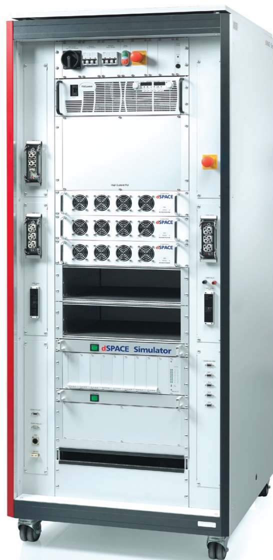
dSPACE Simulator with the highly dynamic load emulator DS5381 (center).
