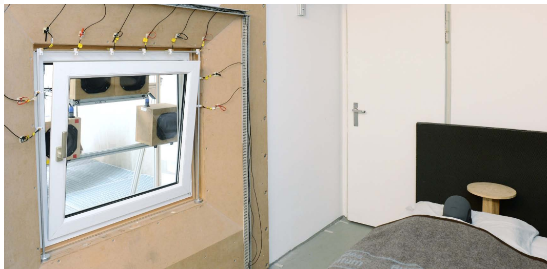
Figure 1: Noise-cancellation speakers reduce the noise before it reaches the window (third project phase).
