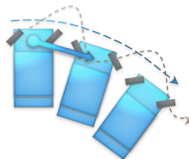
Figure 1: Example of a side maneuver to the right: The vehicle automatically moves in "indirect" motion mode when the position of the joystick is kept to the right.
