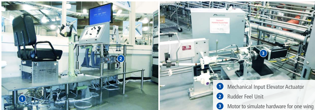
Figure 8: Left: Pilot control station with representative controls and related flight control hardware. Right: High lift test rig for commercial flight control systems.
