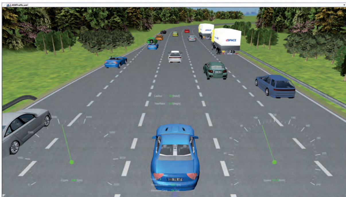
The Road Generator interacts with MotionDesk, the 3-D animation software, to produce realistic visualizations of simulated driving scenarios.
