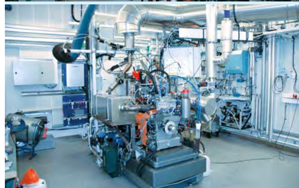
AVL Raptor including a dSPACE system can control, for example, a single-cylinder test bench for gasoline engines with a fully flexible valve system.
