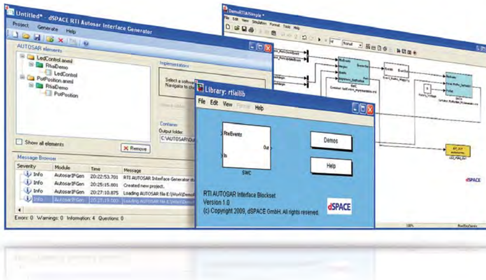
Work in the familiar MATLAB/Simulink environment: Import AUTOSAR software components, and combine them with Simulink and RTI blocks.
