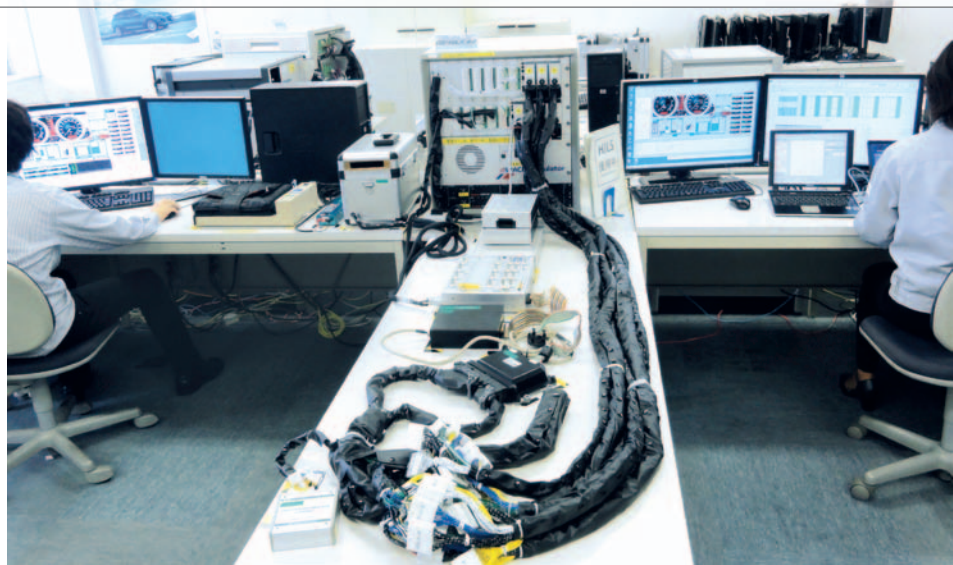
Figure 5: Test bench for the SKYACTIV-G ECUs.
