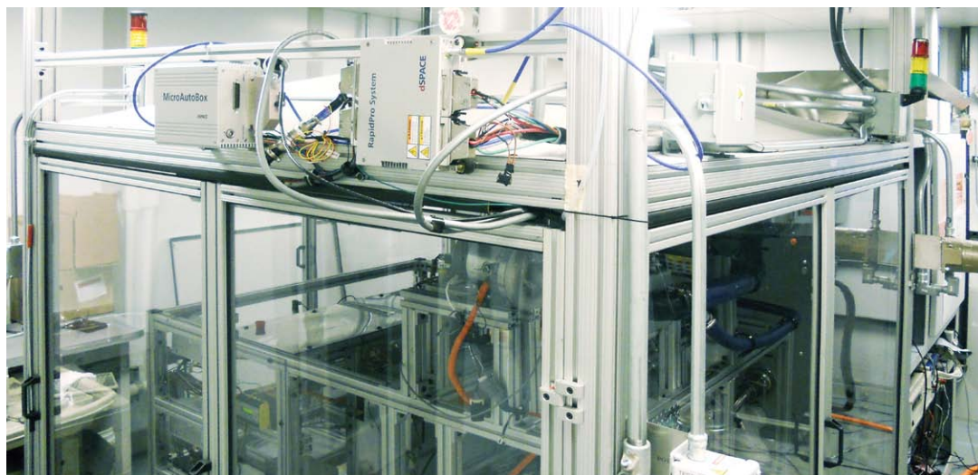
Figure 3: Lab setup of the fuel cell system with MicroAutoBox and RapidPro.
