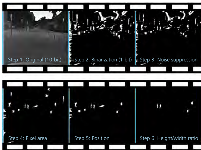
Candidates for spotlighting are detected in several image processing steps.
