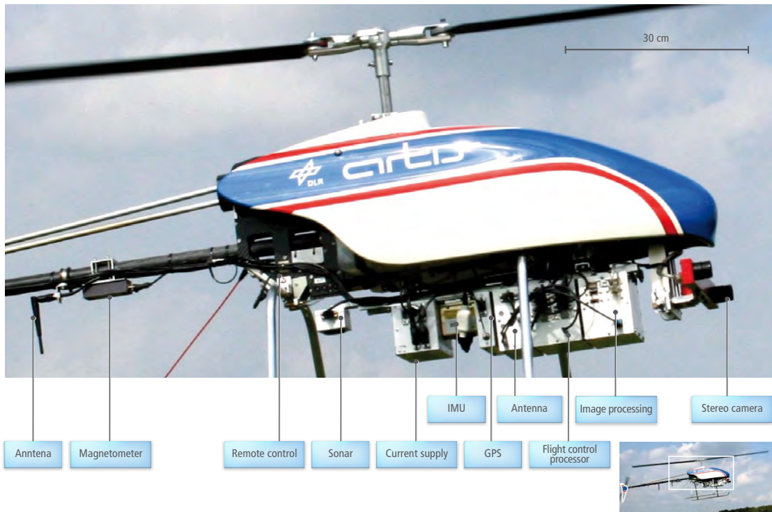
DLR's research UAVs (like ARTIS here) contain numerous onboard systems. These are used for stabilization, flying preset trajectories, automatic take-off and landing, and so on.
