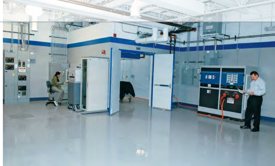
The test chambers are equipped with robust safety and filtration systems – ideal for working with cells and packs using unvalidated support systems.
