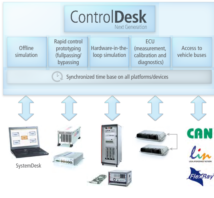
Figure 2: ControlDesk Next Generation, the new universal, scalable experiment tool for ECU development.
