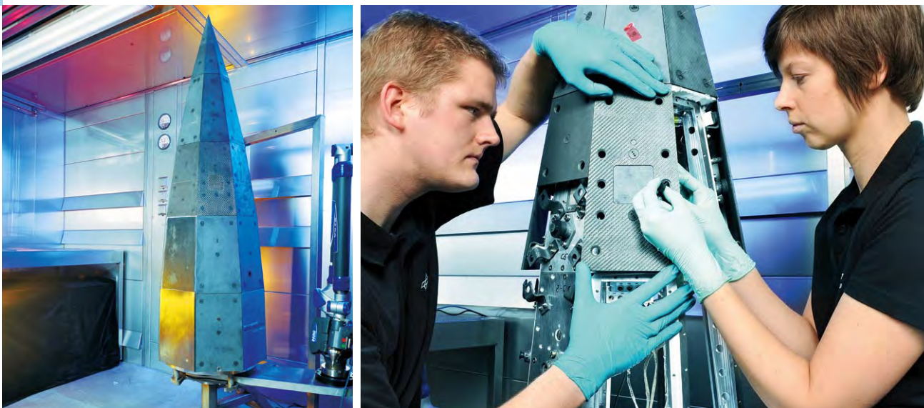
Figure 1: Left: The payload nose cone is just over 2 m long and has flat thermal protection panels. Right: Mounting the panels. Underneath the panels lie temperature sensors, pressure sensors and other devices for in-flight measurements.
