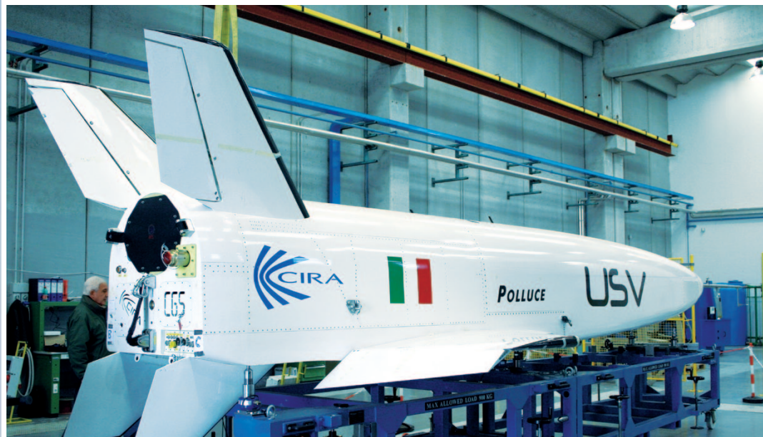
Figure 1: The approx. 9 m long USV glides powerlessly back to Earth, guided only by an onboard computer.
