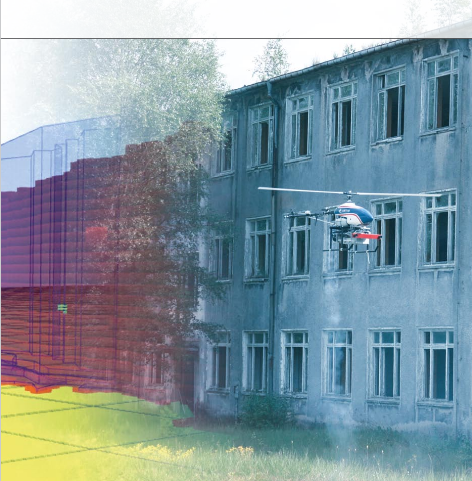
World modeling and mapping in real time during fully automated flight over unknown terrain.
